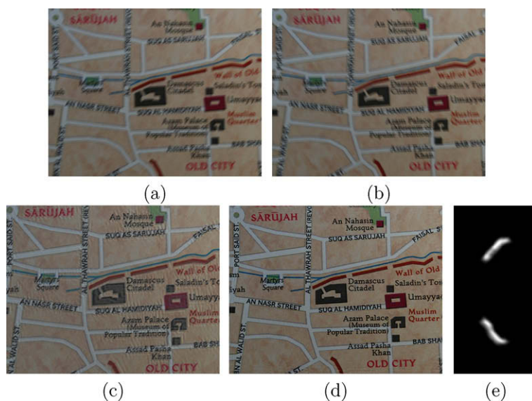
Fig. 8. (a)–(b) two blurred images. (c) The recovered image using the method in [16]. (d) The deblurred image using Algorithm 2. (e) The two blur kernels estimated by Algorithm 2 w.r.t. (a) and (b).
